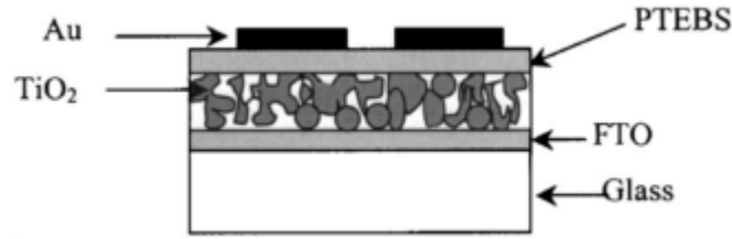
Figure 33. Schematic of bilayer heterojunction hybrid solar cell with configuration of glass/FTO/TiO 2 /PTEBS/Au [40].
